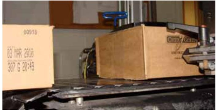
The Videojet 2300 Series printer recycles ink used for automatic printhead maintenance and uses it for printing after filtration. Robinson appreciates that the ink is not wasted and estimates that Golden State Foods can print on thousands of boxes from each can of ink. Plus, the cans are easy to install, and all of the Videojet printers at Golden State Foods require the same type of ink, eliminating the possibility of installing the wrong type of fluid in a printer.
